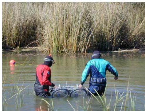
Chemical oceanographers deploy benthic chambers to measure mercury flux in the SF Bay Delta Complex
