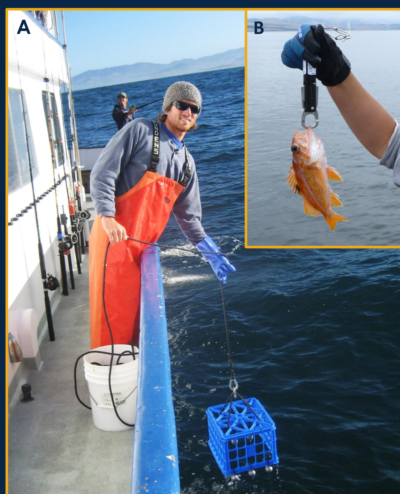
Photo 2. Devices used to descend fish with barotrauma: A. Weighted crate B. SeaQualizer - releases fish at a set depth.
