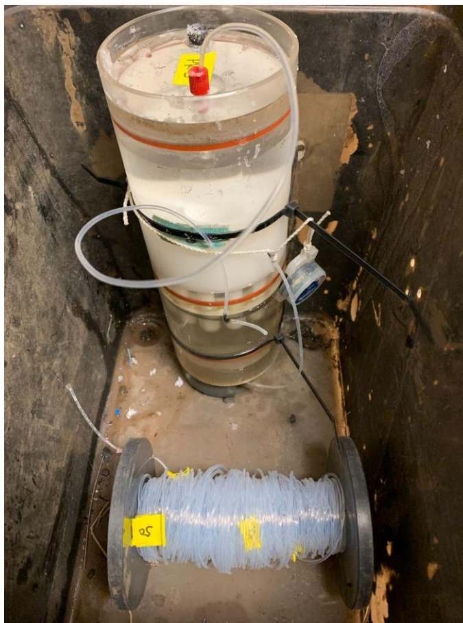
Figure 13. OSMO sampler with 50 m of tubing attached to collect water over a month's time.
