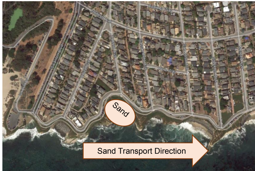
Figure 10-28. Potential sand placement program location at Pyramid Beach with longshore transport direction shown in the arrow, with the intent to nourish and enhance downcoast beaches and offset some of the secondary impacts of coastal armoring.
