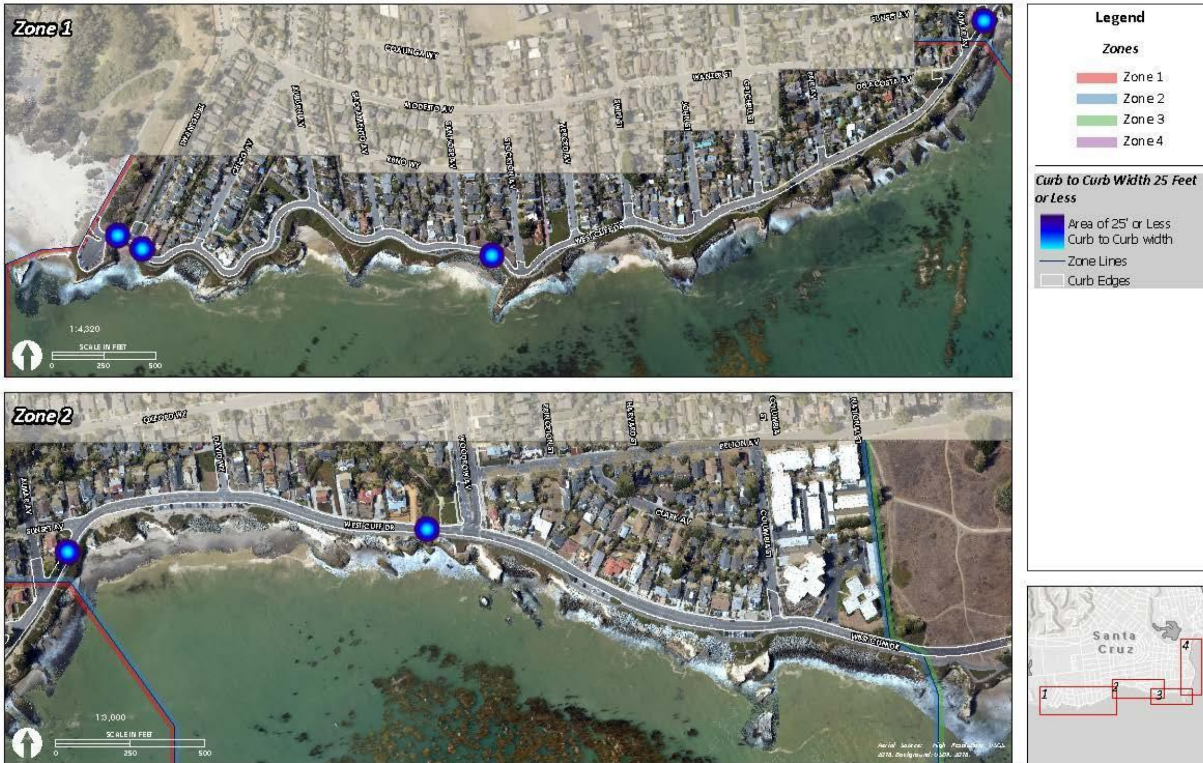
Figure 10-36. Western zones of West Cliff Drive with curb-to-curb ROW width of 25 ft or less.
