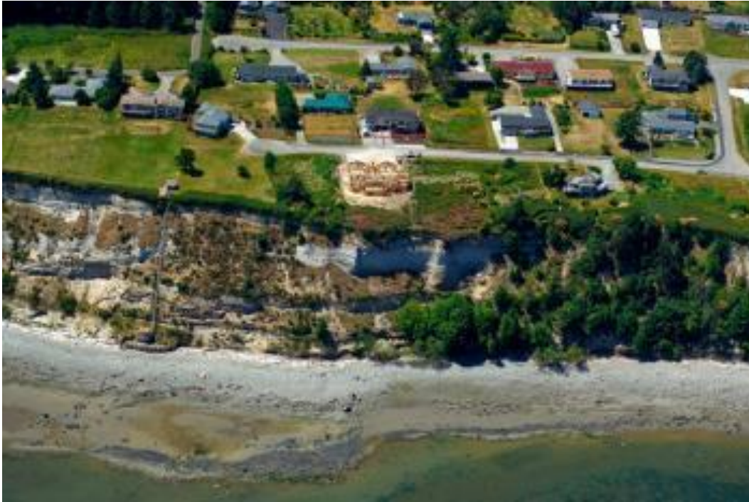
Figure 10-24. Example of setback where development has been moved to inland side of the road near Pismo Beach.
