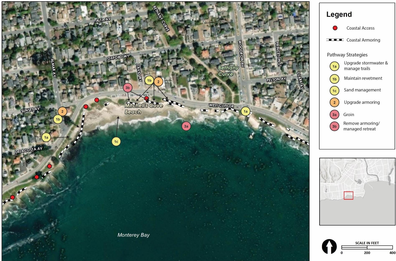
Figure 68. Map showing potential locations to implement strategies within the West Cliff Drive Zone 2 (Mitchell's Cove) adaptation pathway
