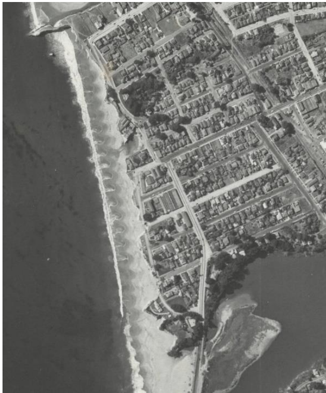
Figure 27. 1953 historical photo shows narrow beach width and bluff erosion at Seabright Beach. source: UCSC Digital Commons
