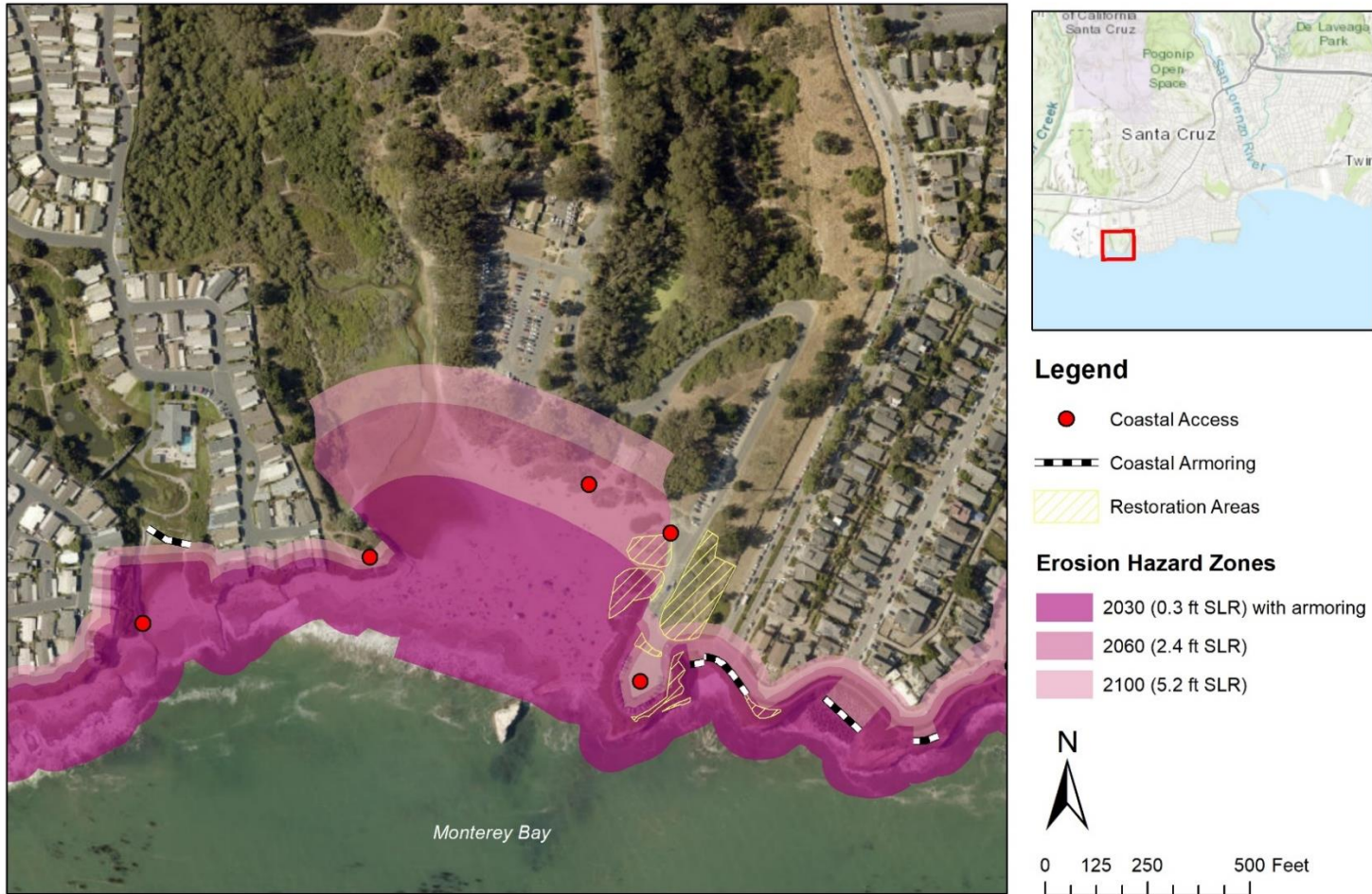
Figure 38. Coastal erosion hazard zones at Natural Bridges Beach for time horizons 2030 (.3 ft SLR), 2060 (2.4 ft SLR), and 2100 (5.2 ft SLR). Existing armoring is accounted for (restricting erosion) through 2030 but assumed to fail to restrict erosion past that time horizon.
