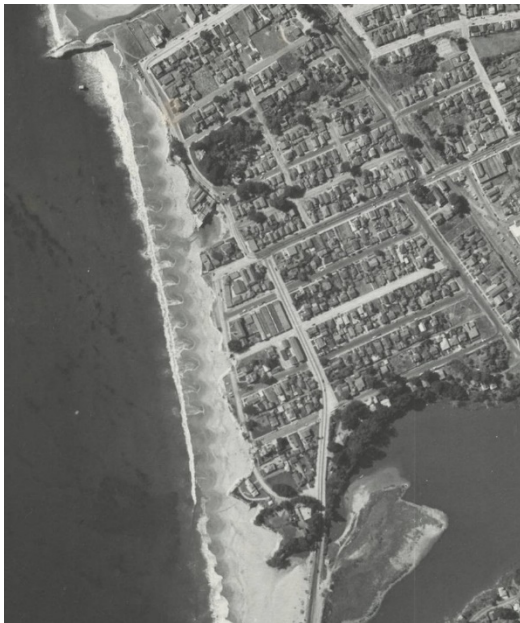
Figure 5. 1953 historical photo shows narrow beach width and bluff erosion at Seabright Beach. source: UCSC Digital Commons
