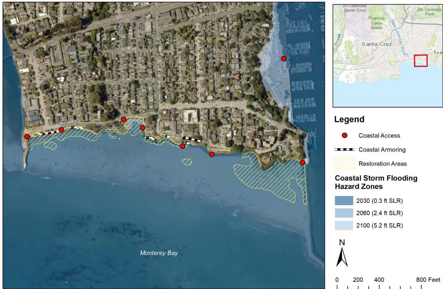
Figure 7. Coastal storm flooding hazard zones at Seabright Beach for time horizons 2030 (0.3 ft SLR), 2060 (2.4 ft SLR), and 2100 (5.2 ft SLR).
