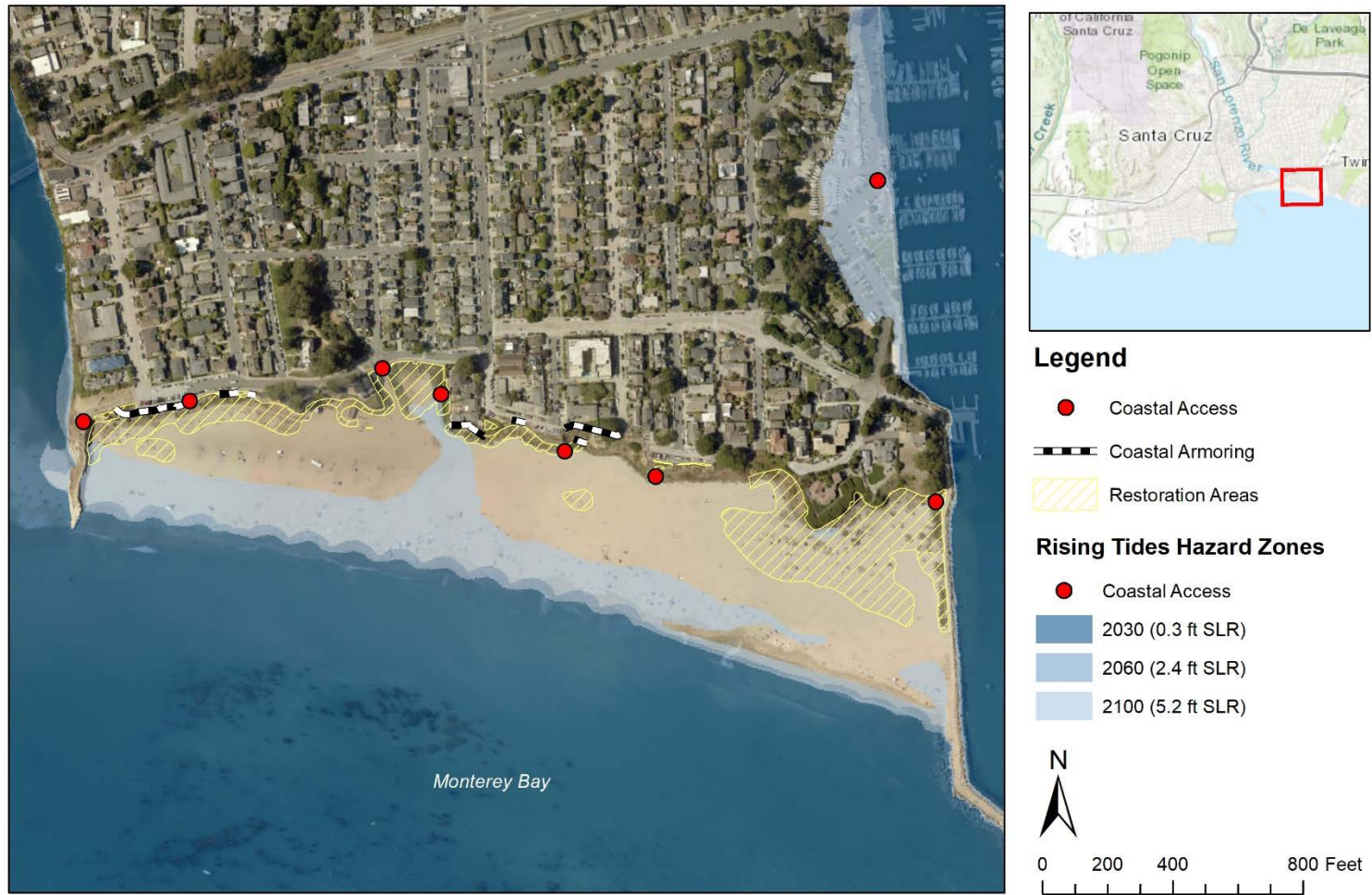
Figure 6. Rising tides hazard zones at Seabright Beach for time horizons 2030 (0.3 ft SLR), 2060 (2.4 ft SLR), and 2100 (5.2 ft SLR).
