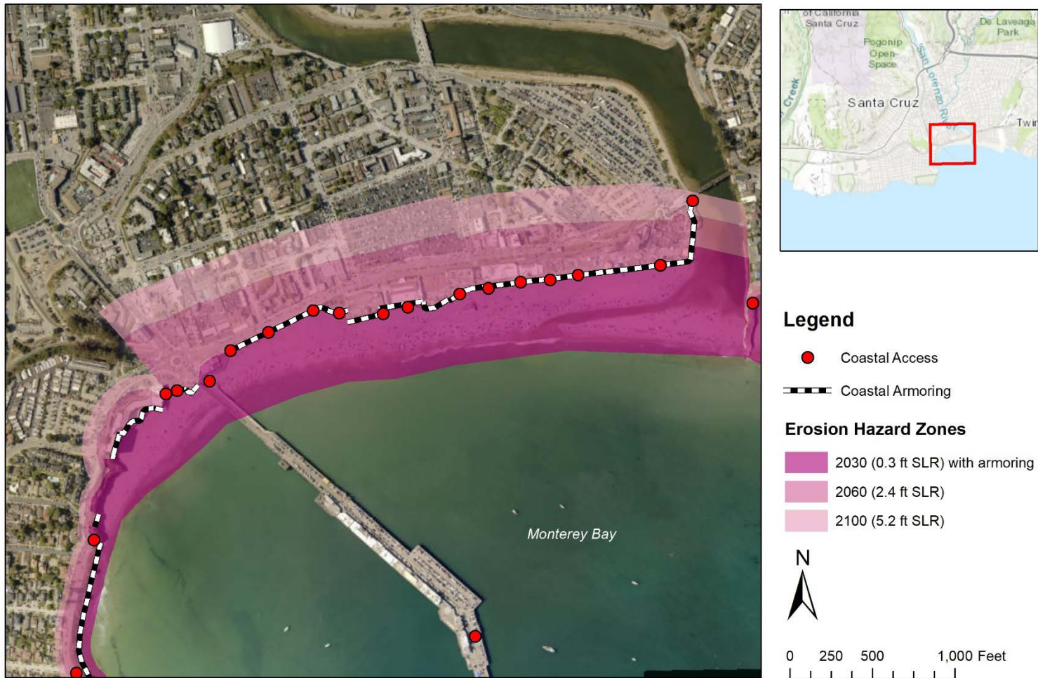
Figure 16. Coastal erosion hazard zones at Main and Cowell Beaches for time horizons 2030 (.3 ft SLR), 2060 (2.4 ft SLR), and 2100 (5.2 ft SLR). Existing armoring is accounted for (restricting erosion) through 2030 but assumed to fail to restrict erosion past that time horizon.
