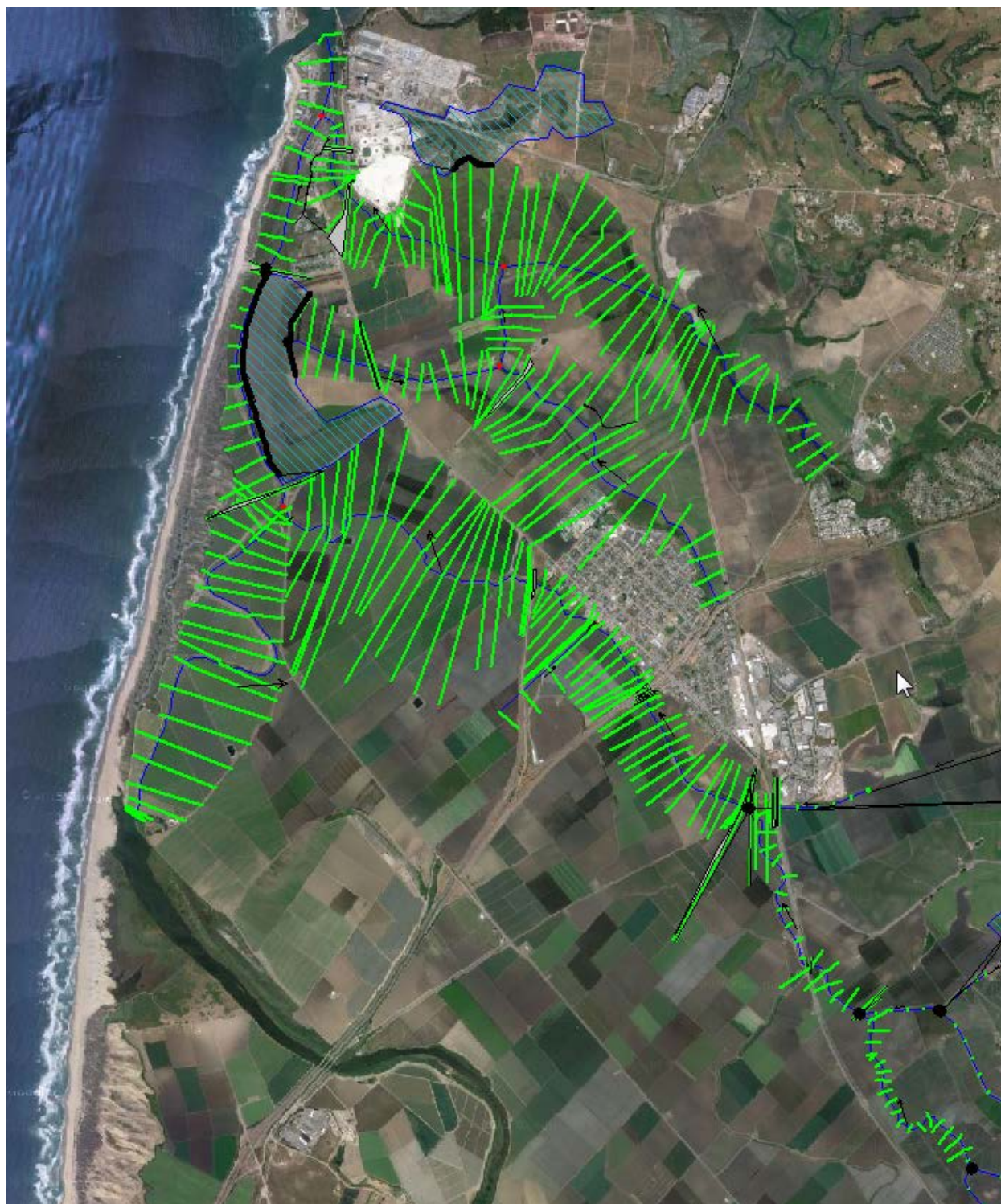
Figure 8. Reclamation Ditch hydraulic model layout
