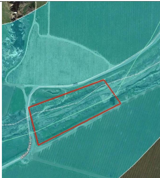
Figure 6d. A non-confined valley where both sides of the river have development within the 100-year floodplain in the form of agricultural fields.
