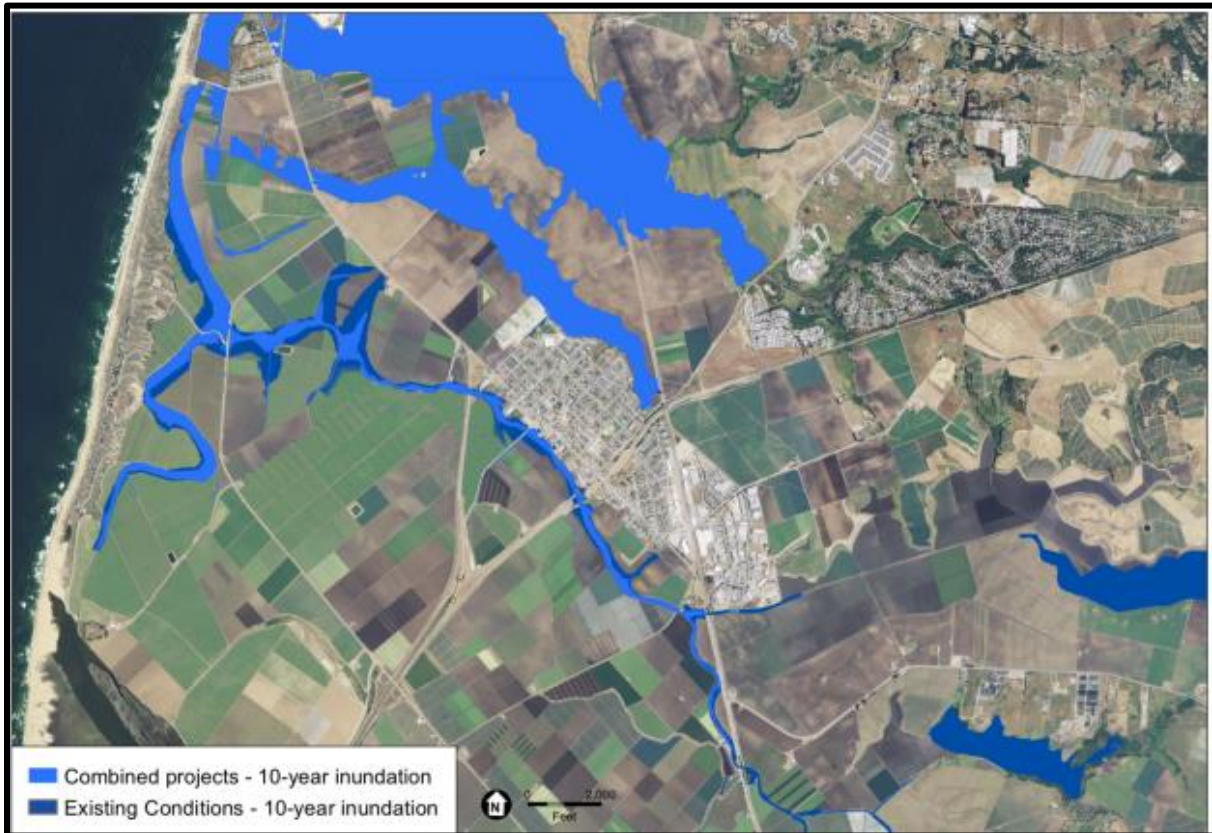
Figure 5. From the 2019 IRWMP Storm Water Resource Plan – predicted 10-year inundation levels in the lower Salinas Valley in a mitigated scenario (light blue) from the cumulative projects and an unmitigated scenario (dark blue) with current conditions.
