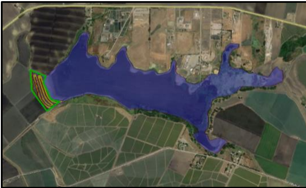
Figure 2A. Espinosa Lake water coverage with five-foot elevation storage extent. The green polygon to the west of the lake is the 10-acre parcel that will be used for seasonal flooding and treatment channels.
