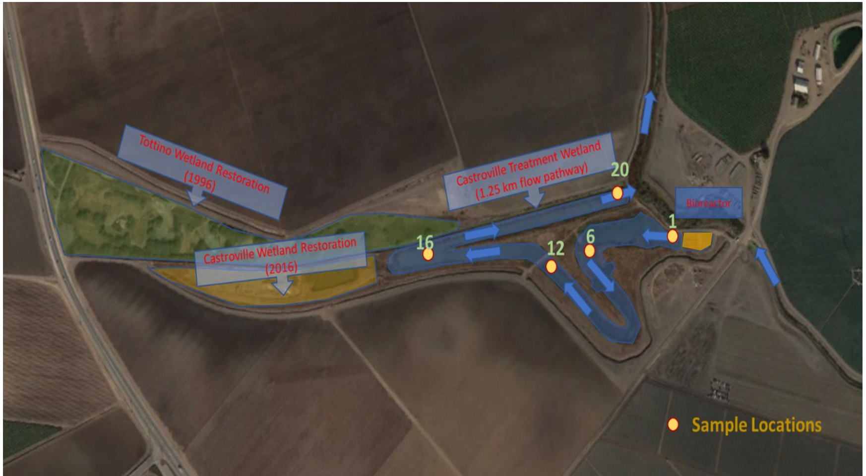
Figure 5. Map of Castroville treatment wetland in relation to watershed flows and adjacent habitat restoration areas. Blue arrows depict flow pathway and yellow dots represent location of a portion of water quality sample sites. The multi-chamber bioreactor research area is located directly upstream of sample location 1.
