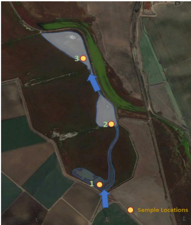
Figure 4. Sea Mist treatment wetland design and sample locations.
