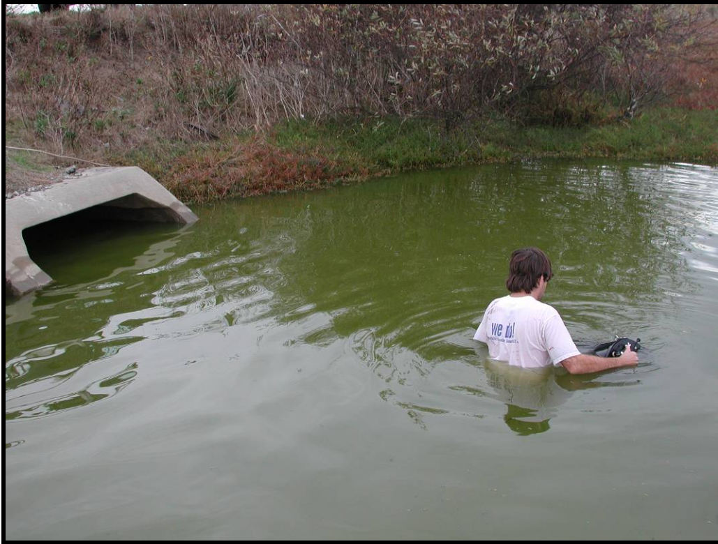
Figure 4. Placing the YSI automated data loggers in the Moro Cojo Slough.
