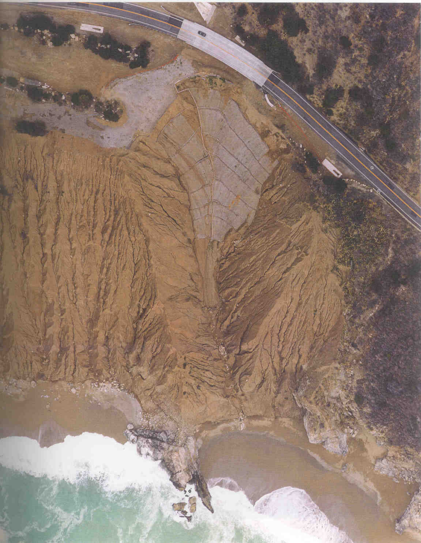
McWay landslide on November 21, 1997 Jute and haybale rows with irrigation pipes Hay, seed, no nutrients except green patches near the bridge
