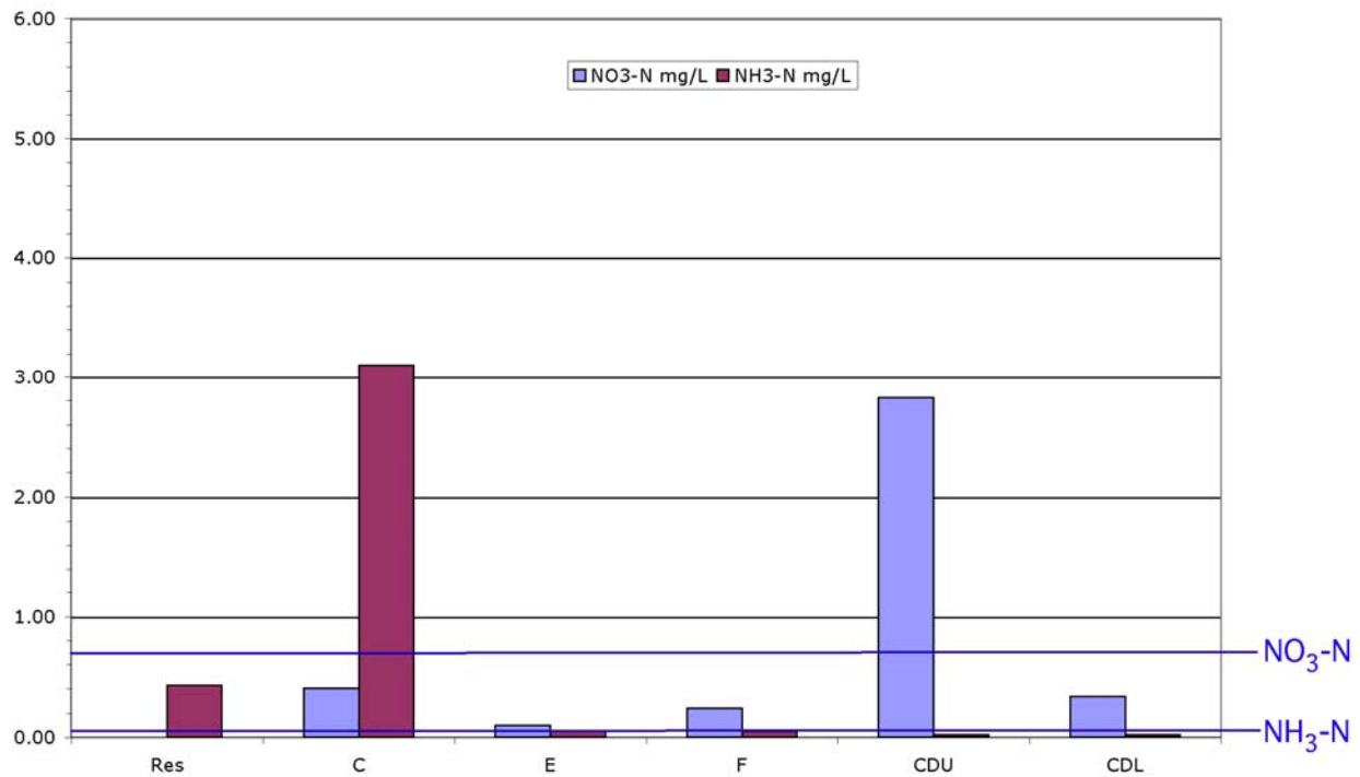
Figure 24. April mean nitrate (NO 3 -N mg/L) and mean total ammonia (NH 3 -N mg/L) concentrations as water flowed from Pond C through the series of ponds to lower Central Ditch, and comparative threshold levels in blue (N = 27).
