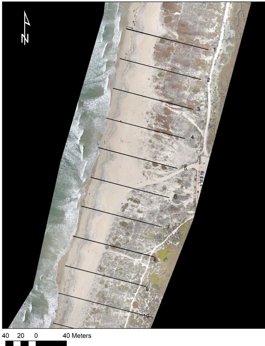
Figure 17. Imagery from UAV survey (2016). The lines represent the locations of cross sections used to assess topographic change for both unrestored areas and restored areas at the Potrero restoration site.
