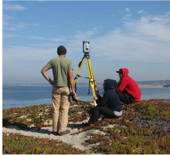
Dr. Ivano Aiello and students surveying the dunes with the terrestrial laser scanner.
