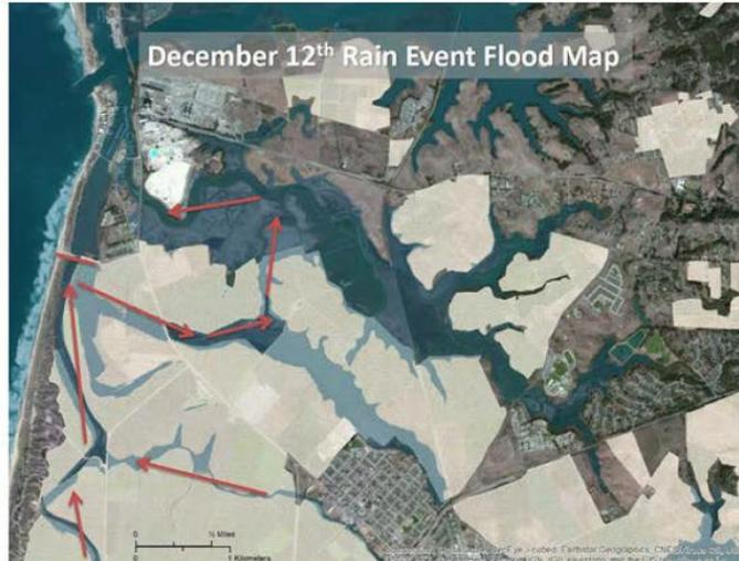
Figure 14. Comparison of Modeled 100-year flow paths and observed flow paths during Dec 2014 flood (Figure source: ESA 2014)
