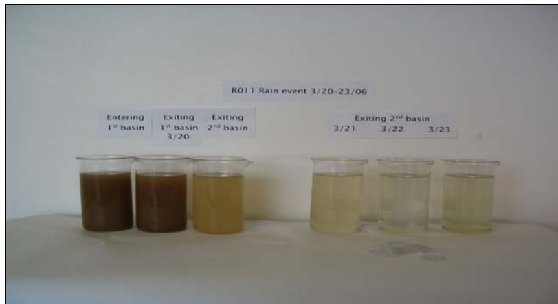
Figure 9.14. R011 Suspended sediment samples from the 3/20–24/06 rain event.
