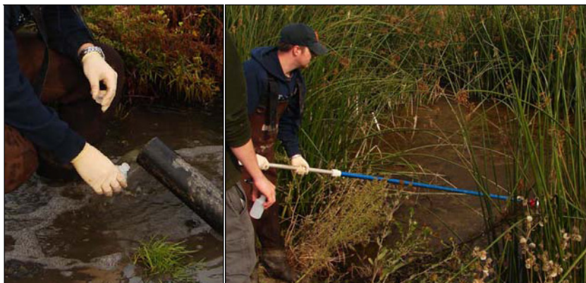
Figure 13.4. Taking nutrient samples at the upper Wetland exit (DCR-003) and the mid-point of the upper section (DCR-002). Photos: Brianne Bieschke, 2006.
