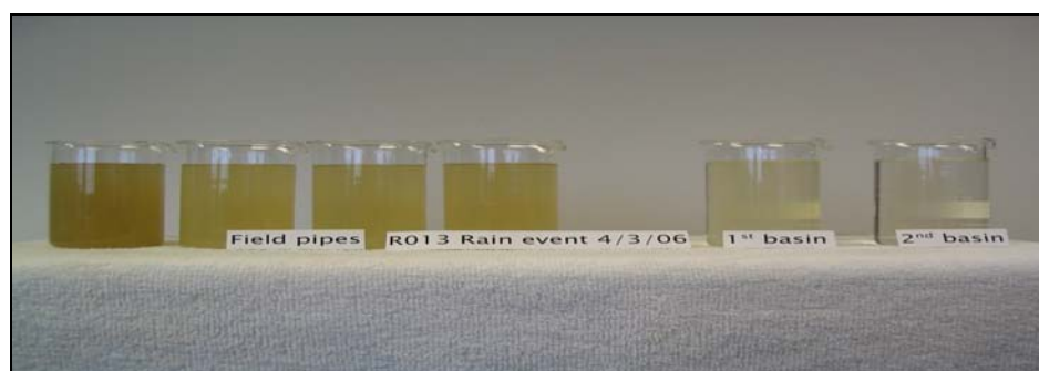
Figure 9.15. R013 suspended sediment samples for 4/3/06.
