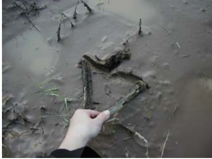
Figure 9.11. Fine sediment captured in Basin 1.
