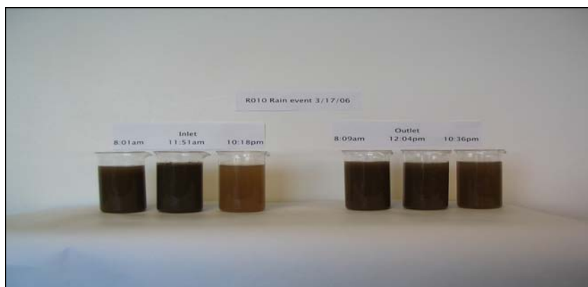
Figure 9.13. R010 suspended sediment samples from the 3/17/06 rain event.
